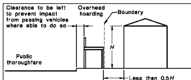
The Principal Contractor or Owner-builder must ensure that overhead protective structures are installed and maintained in accordance with the NSW “Code of Practice - Overhead Protective Structures 1995”. This is code available at [www.safework.nsw.gov.au/data/assets/pdf\\_file/0008/52883/Overhead-protective-structures-Code-of-practice.pdf](http://www.safework.nsw.gov.au/data/assets/pdf_file/0008/52883/Overhead-protective-structures-Code-of-practice.pdf)
